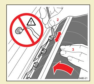
Rotate the drum away from you (toward the back of the printer); this rotates the clamp rollers. Clean the entire surface of the roller.
